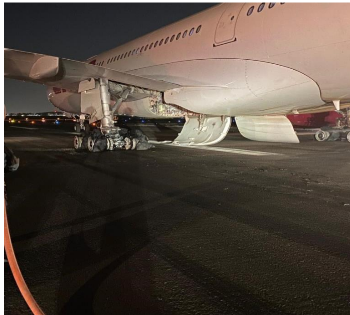
Figure 4 All Tires burst after the aircraft came to a stop.
