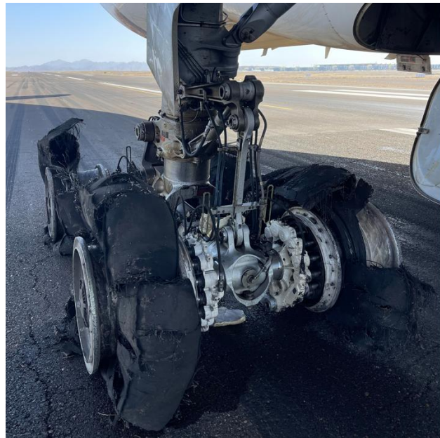
Figure 7 Remanent of the Right gear tires.
