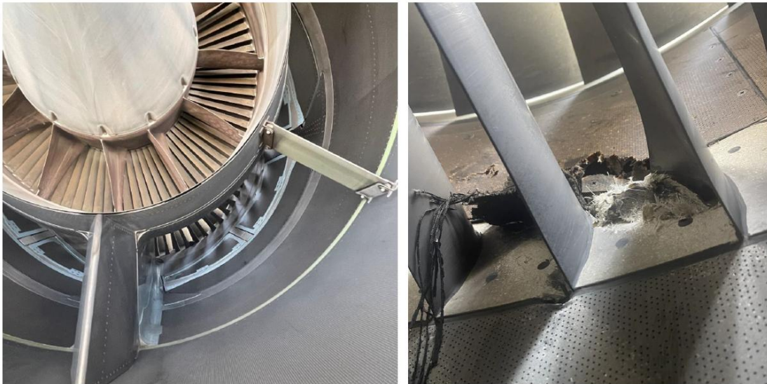
Figure 13 L/H engine aft Fan blades acoustic panel damaged (caused by tire rubber).
