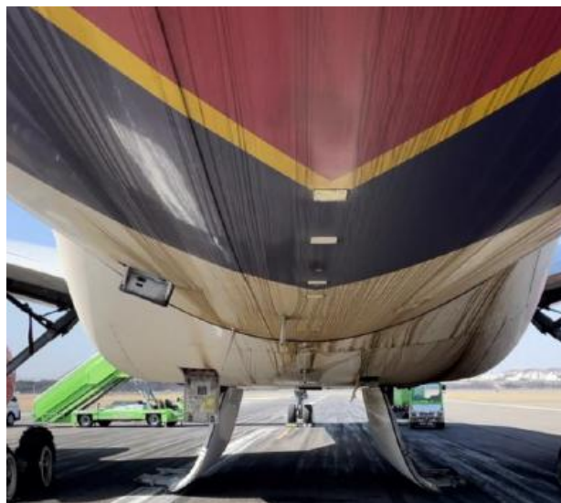
Figure 8 Main Gear doors touching the ground, showing a hydraulic fluid stain.
