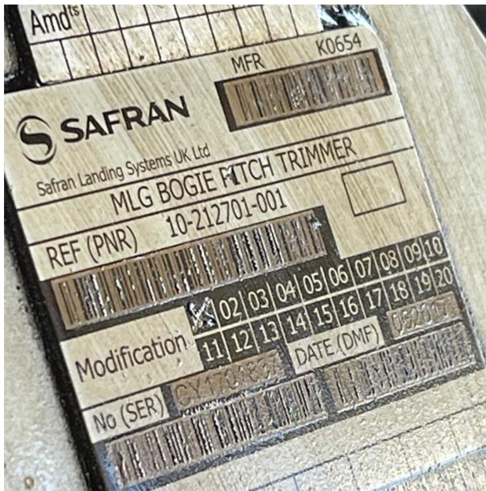
Figure 24 R/H Trimmer Actuator data plate
