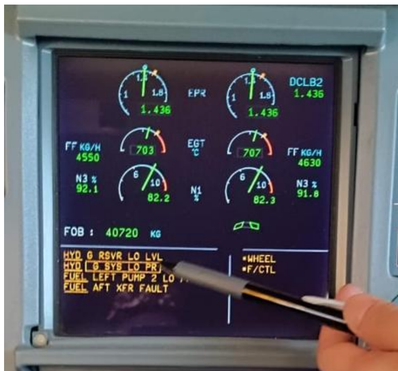
Figure 1 In-flight ECAM display of Green HYD system loss.
