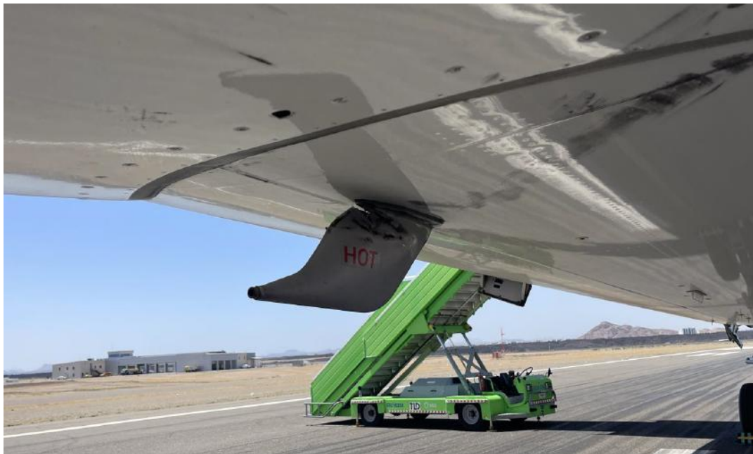
Figure 11 Damaged FWD water drain mast.
